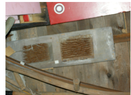
* Hackler Drawn through wool to rough grade wool for carding
